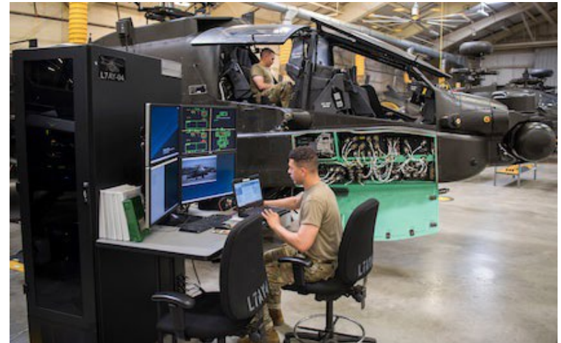
Photo: U.S. Army Pvt. Cameron Guy reads a systems console for a Boeing AH-64 Apache attack helicopter simulator, while fellow student U.S. Army Pfc. Brady Peckinpaugh reviews the reading from the cockpit at Joint Base Langley-Eustis, July 22, 2022. (U.S. Air Force Photo by Abraham Essenmacher).
